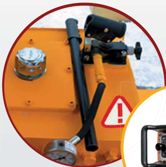
Emergency Hand Pump
